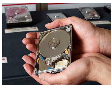
Hitachi, TOSHIBA HDD (perpendicular magnetic recording)
